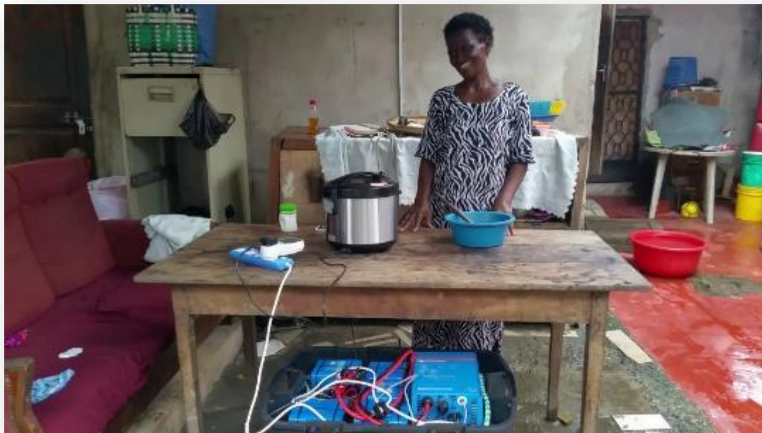
Figure 29: 'Under-the-table' mode (with lid off for the photo), allowing the cook to use the prototype as if the appliances were connected to the grid.
