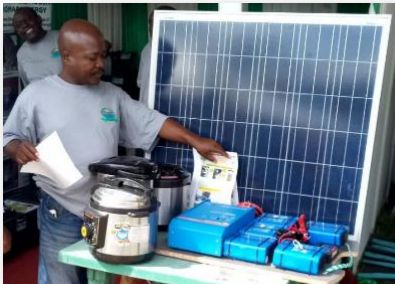
Figure 26: Photos of eCook TZ Mark 1 Prototype key components (before the wiring was tidied up!).
